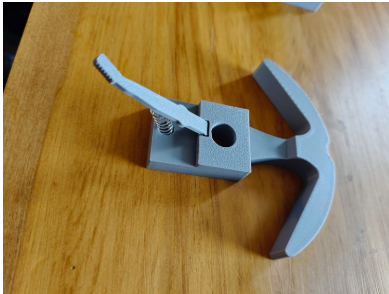
Swing arm assembled with spring loosely in place
